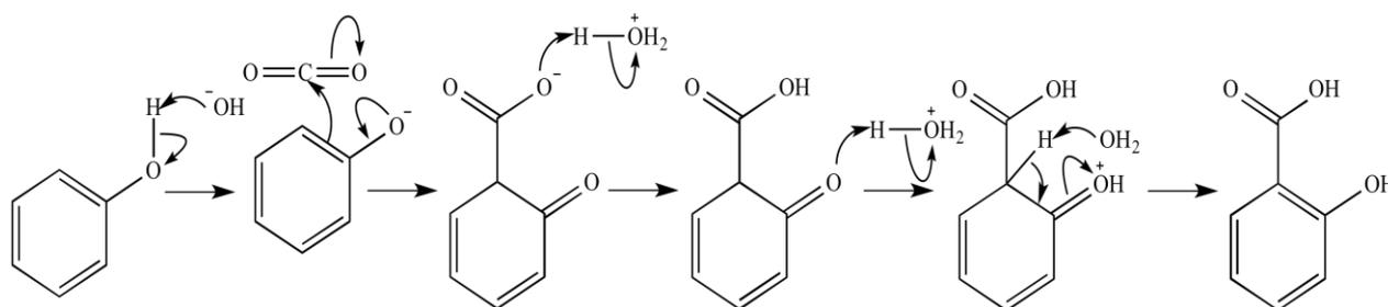
Fig. 2: Salicylic acid production by Kolbe – Schmitt reaction [35]
