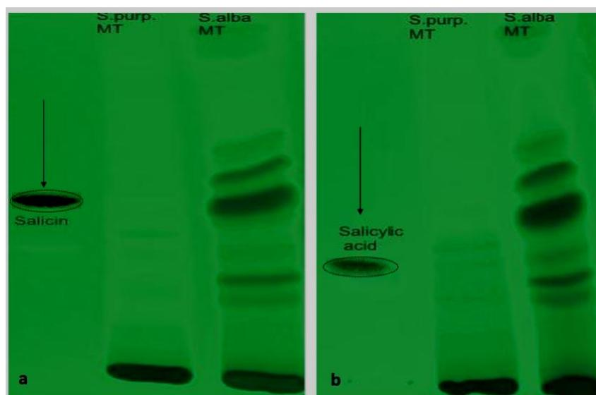
Fig. 3: The TLC chromatograms in UV 254 nm salicin (a), salicylic acid (b)
